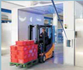
Enclosure IP-55 with toughened glass door for RFID Reader
